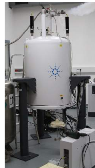
NEW 600 MHz Agilent DD2 spectrometer equipped with ^1\text{H} and ^{13}\text{C} enhanced triple resonance salt tolerant (HCN) cryogenic probe head
