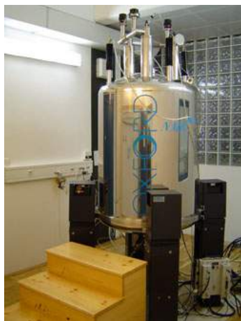
600 MHz Varian VNMRS spectrometer equipped with wide range of solid-state and liquid probe heads
