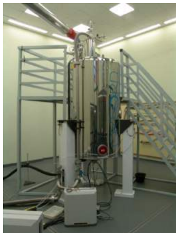
800 MHz Varian VNMRS spectrometer equipped with ^1\text{H} and ^{13}\text{C} enhanced triple resonance (HCN) cryogenic probe head
