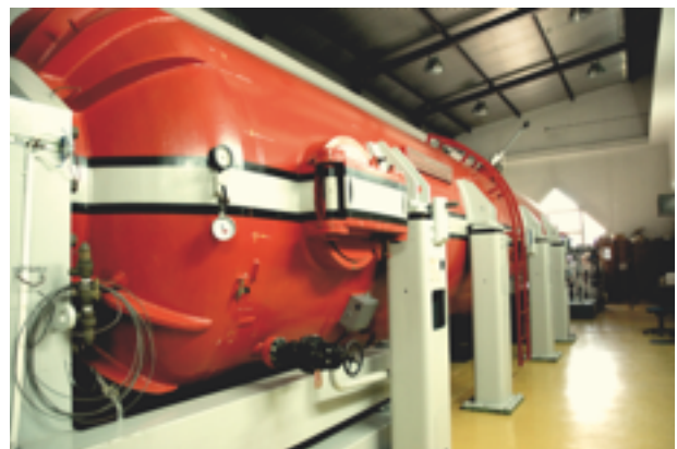
Figure 25 - 6.0 MV EN Tandem Van de Graaff Accelerator at the Ruđer Bošković Institute in Zagreb, Croatia
